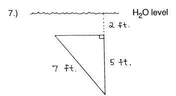
Find the total force due to water pressure on one side of the submerged, triangular (flat) plate.
