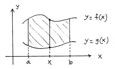
$$\bar{x} = \frac{\int_a^b x (f(x) - (g(x))\delta(x, y) \, dx}{\int_a^b (f(x) - g(x))\delta(x, y) \, dx} \quad \text{and} \quad \bar{y} = \frac{\int_a^b (1/2)((f(x))^2 - (g(x))^2)\delta(x, y) \, dx}{\int_a^b (f(x) - g(x))\delta(x, y) \, dx}$$
