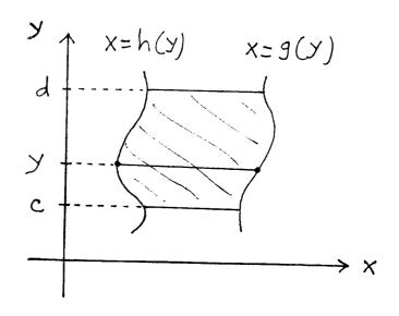
$$\bar{x} = \frac{\int_{c}^{d} (1/2)((g(y))^{2} - (h(y))^{2}) dy}{\int_{c}^{d} (g(y) - h(y)) dy} \quad \text{and} \quad \bar{y} = \frac{\int_{c}^{d} y(g(y) - h(y)) dy}{\int_{c}^{d} (g(y) - h(y)) dy}$$
