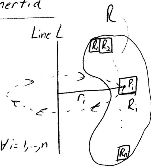
Note: the mass of  $R_i$  is approx.  $M_i \approx \delta(P_i) \Delta A_i \forall i=1, \dots, n$
