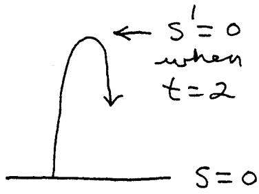
$$\begin{aligned} s(t) &= -16t^2 + v_0 t + s_0 \rightarrow \\ s(t) &= -16t^2 + v_0 t \rightarrow \\ s'(t) &= -32t + v_0 \end{aligned}$$
