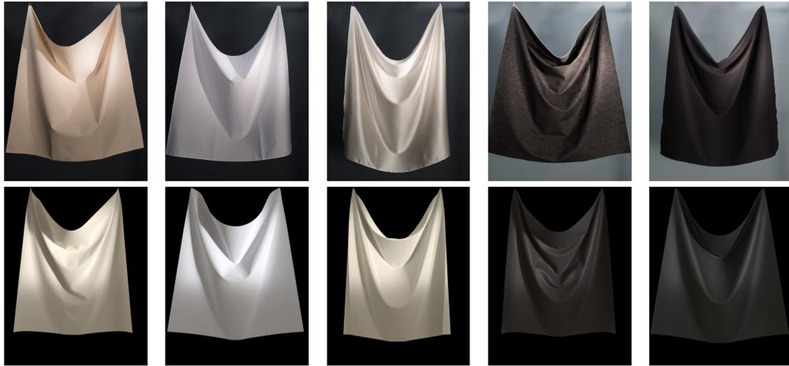
**Figure 1:** Photographs of five fabrics (canvas, cotton poplin, silk charmeuse, denim and wool coating) along with the corresponding simulation after parameter estimation (bottom row). Each piece of fabric is  $1\text{m} \times 1\text{m}$ , and the top corners are held  $60\text{cm}$  apart. The real fabrics had multiple stable equilibria for the specified constraints, so exact matches cannot be expected.
