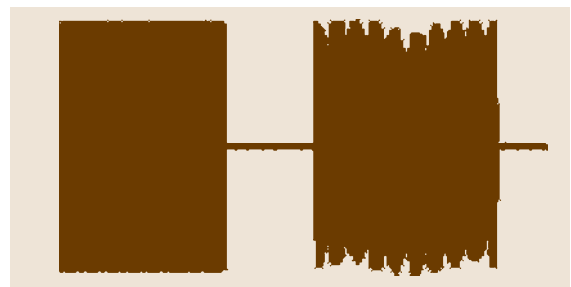
Fig. 15.5 Wave envelope of a major triad chord based on the Pythagorean scale followed by the same chord on the equal-tempered scale, with pronounced beats in the amplitude arising from the departures from harmonicity in the frequencies of the major third and perfect fifth
