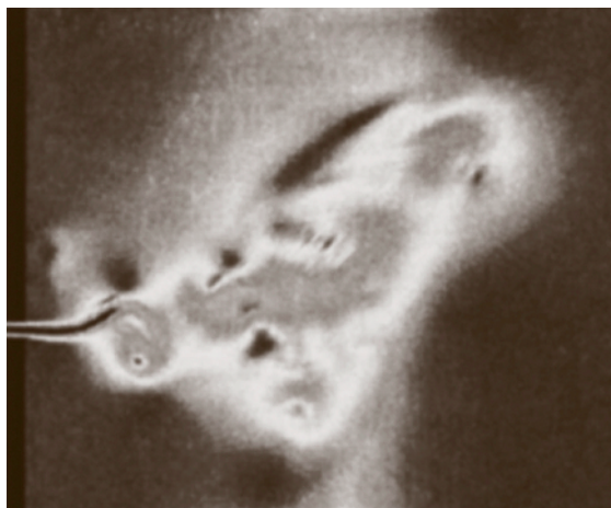
Fig. 15.109 A computed snapshot showing the breakup of a jet and generation of vortices (Adachi [15.184])
