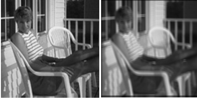
Figure 4.3. Filtered output (right) of color image (left) using Prewitt edge detector (see color section within this book for a full color version of this figure)
