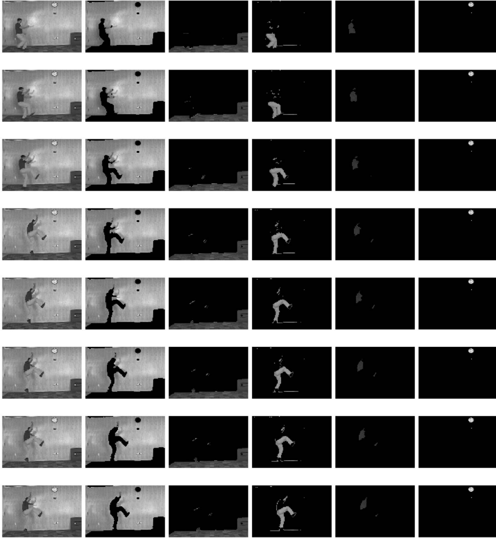
Fig. 9. The leap: The original frames (120 × 80 pixels) are shown in the left column. Each column shows slices through a space-time segment.
