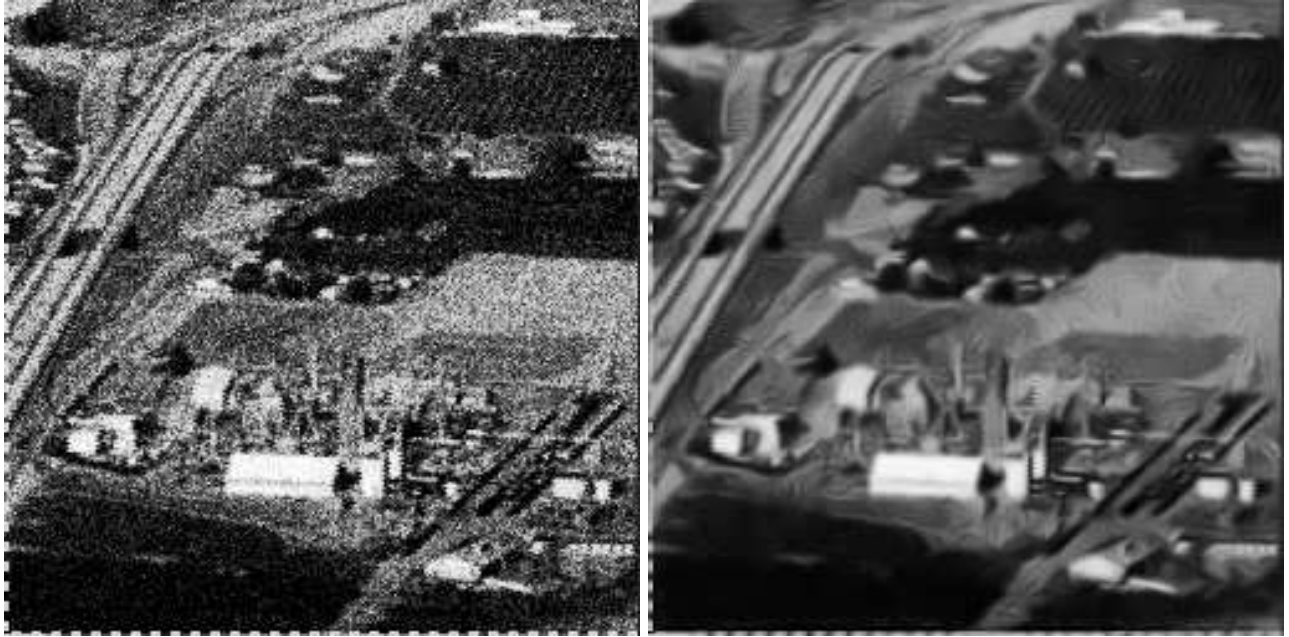
Figure 1. Left: original noisy image. Right: image denoised by application of the Markov matrix as in (1)
