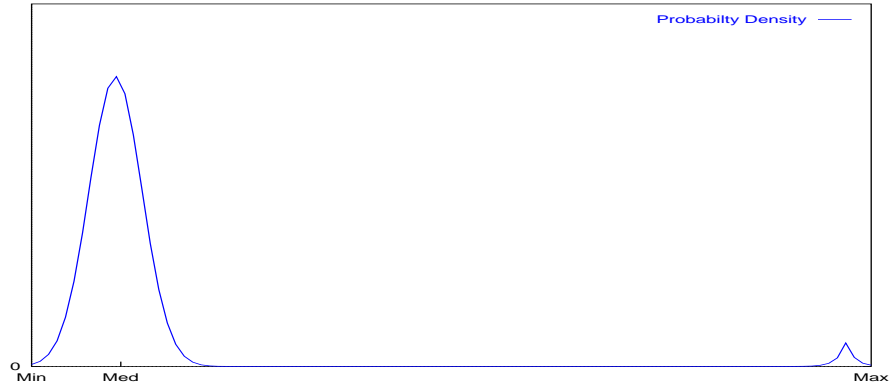
Figure 3.19: Probability density function of a radar image with targets, showing the range of data.
