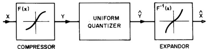
Fig. 6. Companding model of nonuniform quantization.
