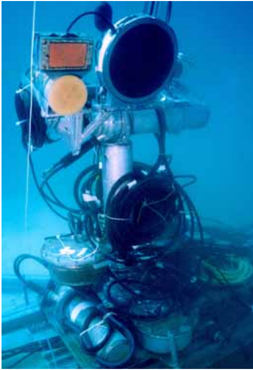
Fig. 4. Photo of transducers on sonar tower.
