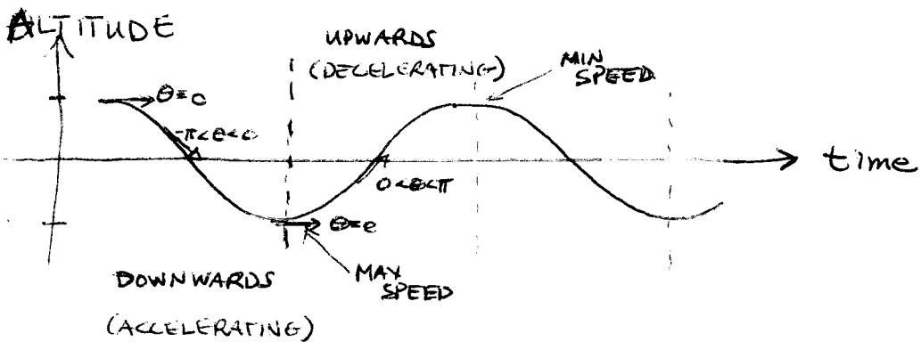
(ii) FIXED POINT corresponds to horizontal flight (at a constant altitude and a constant velocity).
