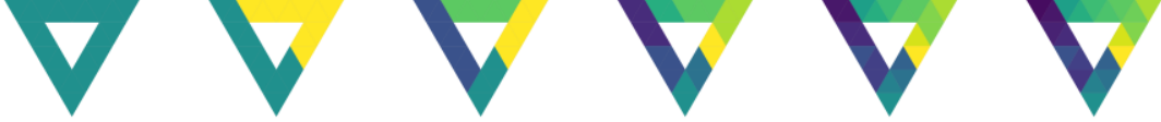
FIGURE 4.7. One possible hierarchical bipartitioning of a simple 2-complex, from j = 0 with no partition on the left, to j = 5 on the right, where each of the 21 triangles form their own subregion. Colors indicate distinct subregions.
