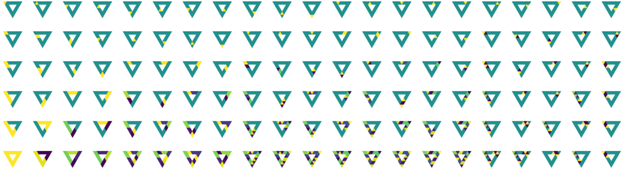
FIGURE 5.4. Fine-to-Coarse (F2C) 2-GHWT dictionary. Note that this dictionary is not generated by simply reversing the row indices of the C2F dictionary, but instead by arranging each level (row) by “sequency”.
