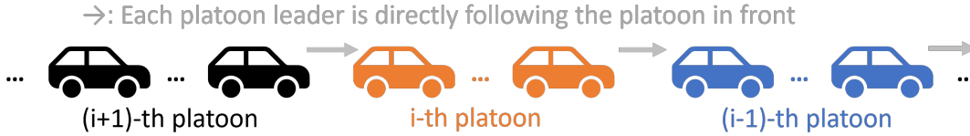
FIGURE 3.3. CF pattern of multiple platoons with no inter-platoon communication.
