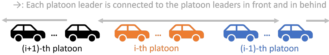
FIGURE 3.4. CF pattern of multiple platoons with forward and backward inter-platoon communication.
